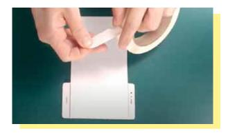
Using a piece of tape, fix the white paper over the screen where you see the shape of the connector. Beware not to cover the mic, camera, or light sensor with the tape, otherwise, the device may stop working properly.
